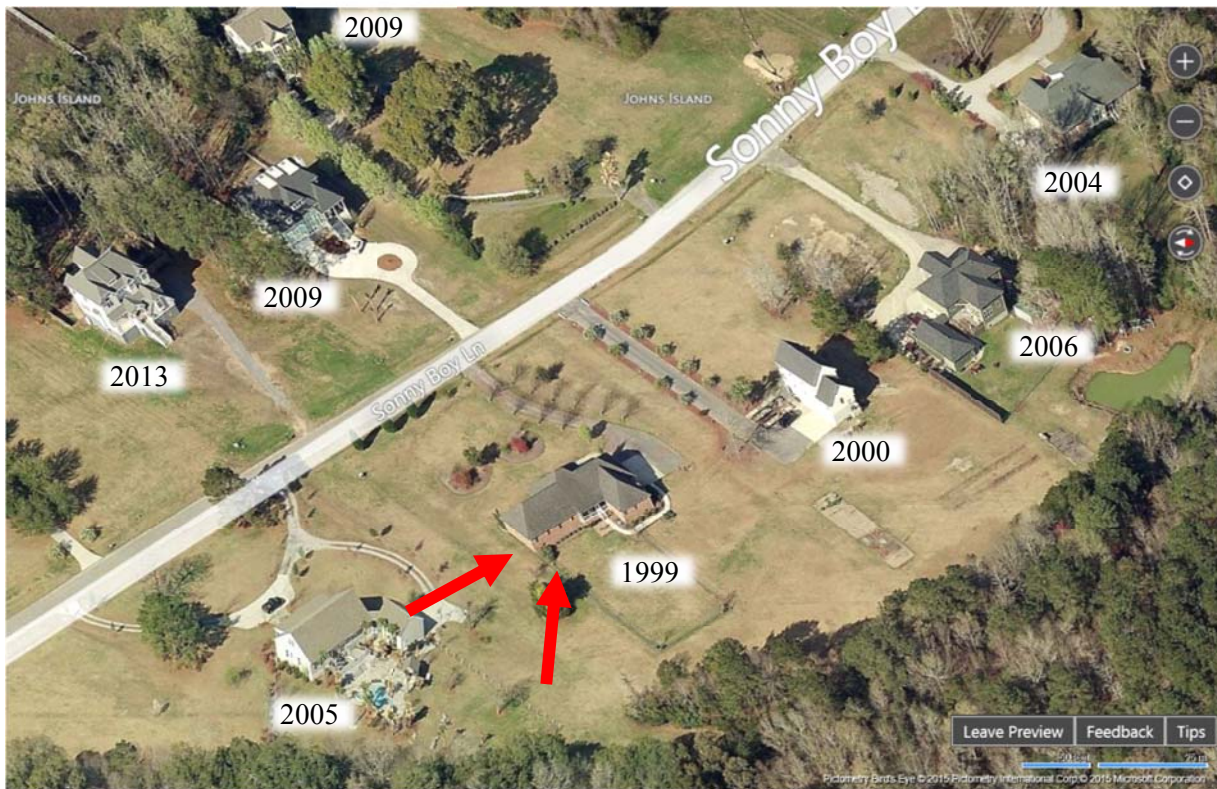
Figure 11: Birds eye view of the destroyed home. Solid red arrows indicate the range of wind directions the home was exposed to during the passage of the tornado based on the debris and treefall patterns (see Figure 7). The white arrow with red outline indicates the approximate direction of travel of the tornado as it passed this area. The exact path of the tornado center is not known however.
