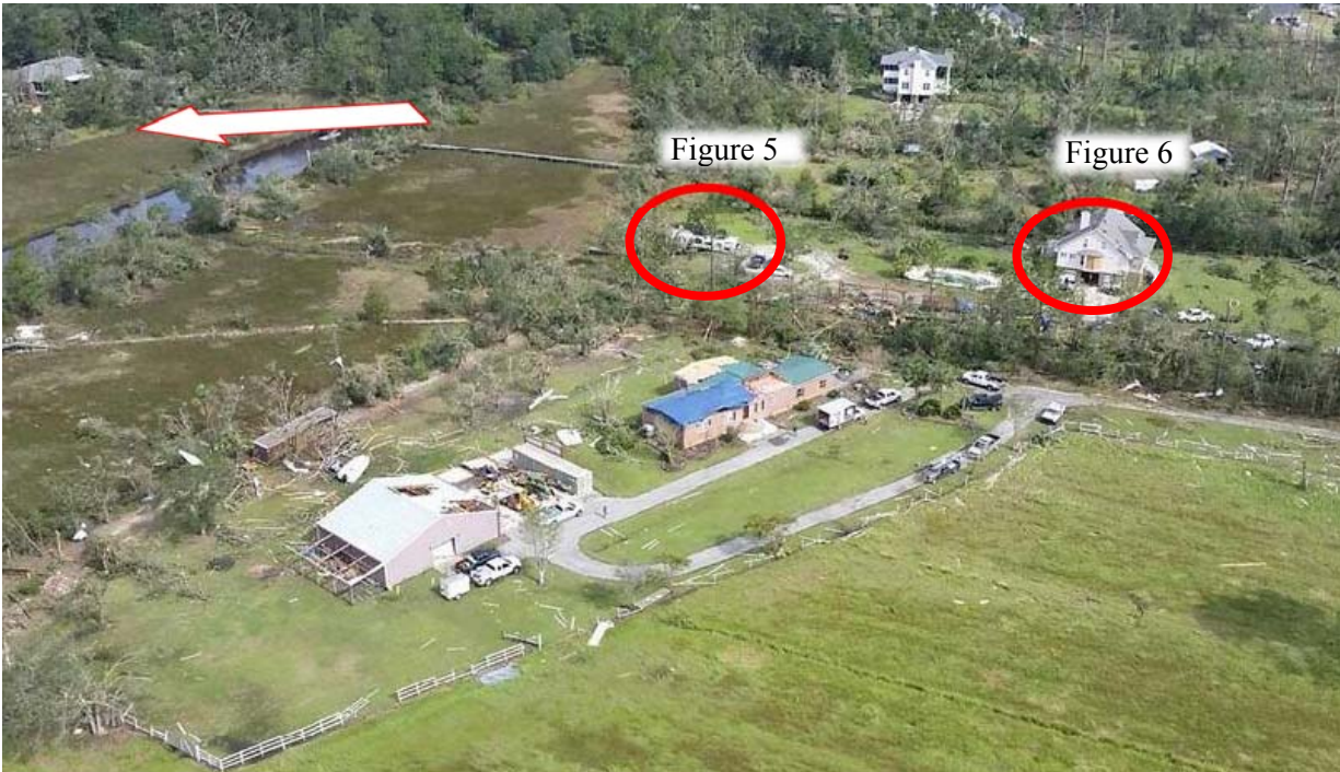
Figure 4: Aerial view of damage along Old Pond Rd. Roof damage was observed to two commercial buildings and a nearby home suffered damage to a bay window, garage door and roof covering. A camper was flipped in the same property. Approximate direction of tornado is indicated by white arrow. (Photo from ABCNews4.com )
