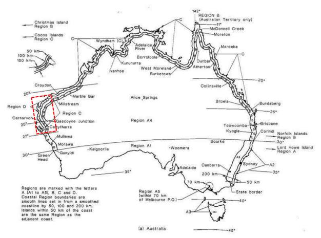
**Figure 3.** Design wind speeds for Australia based upon AS 1170.2 (2002). The region impacted by Tropical Cyclone Olwyn (highlighted by the rectangle) has a design wind speed varying from 88 m/s (316 km/h, 197 mph, V0.2) for Exmouth to Carnarvon in Region D, to 57 m/s (205 km/h, 128 mph, V0.2) at Geraldton in Region B.
