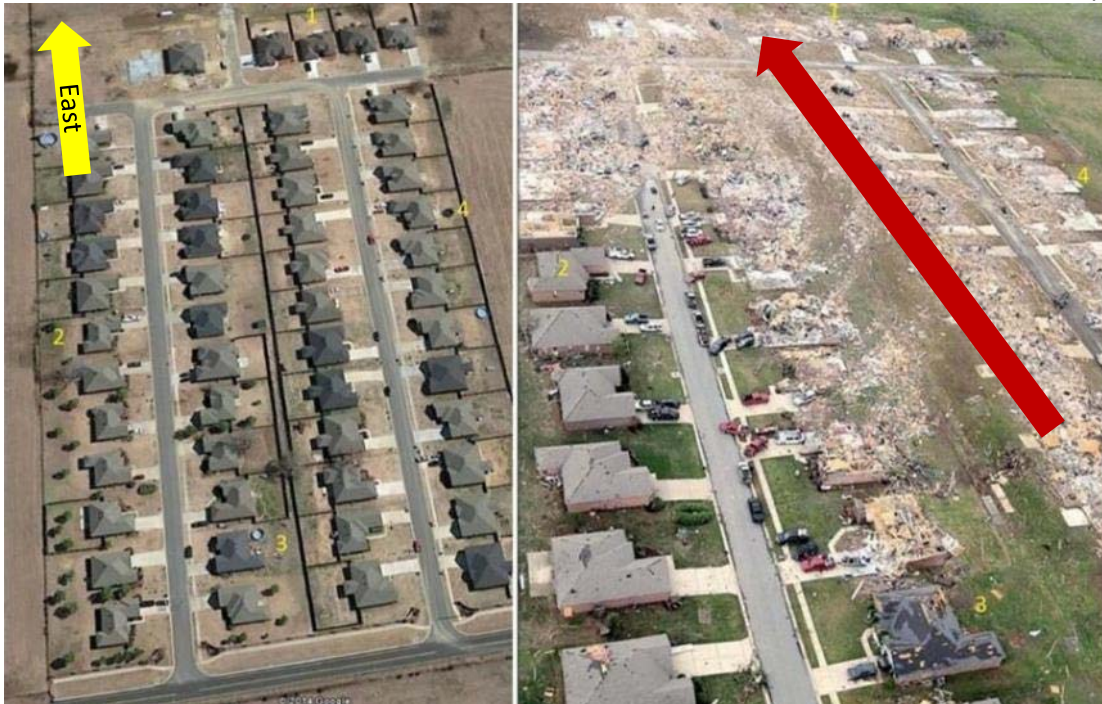
Figure 17. Comparison of Parkwood Meadows subdivision before and after the tornado. The yellow arrow indicates the East direction, while the red arrow indicates the estimated tornado centerline through the subdivision. (Photo Courtesy of Twitter user @Scott_Ar).
