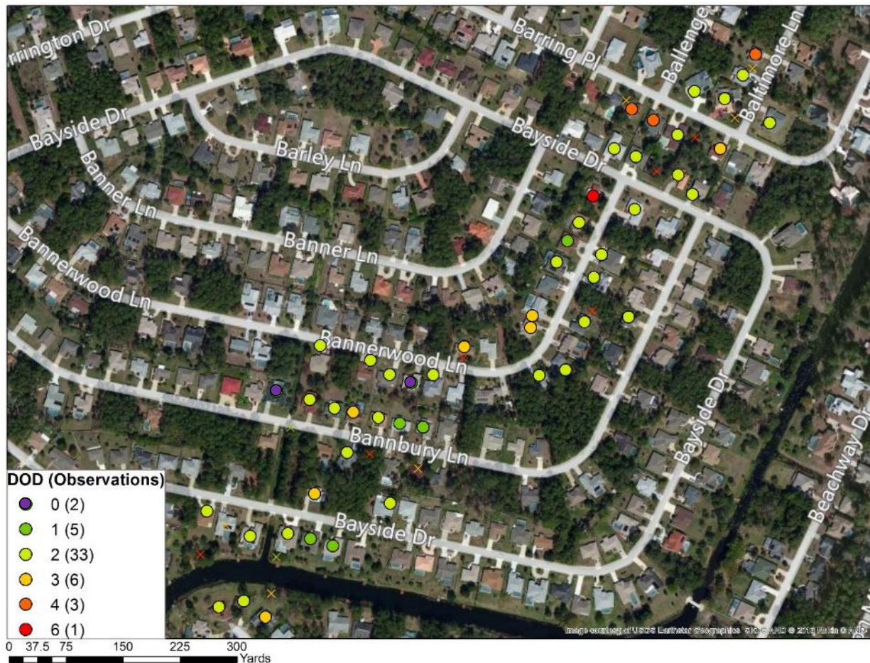
Figure 7: Assigned Degrees of Damage for the homes (solid circles) and tree damage (marked by X) surveyed by the UF WHDA team
